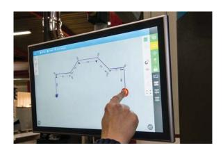
The application of Multi Touch technology reduces the number of keyboard- and button actions to an absolute minimum. The innovative Smart Draft, Design/Bending Sequence Multitasking, Step Previewer and Combined Icons features allow the operator a straightforward, intuitive control of the entire production cycle.
