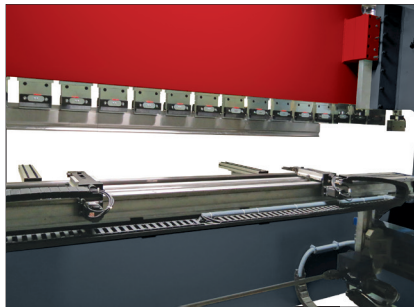
X-R-Z1-Z2 4 axis backgauge (optional)
