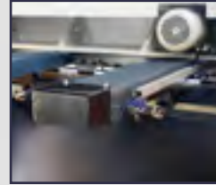
NC Kontrollü, Motorlu 750mm ve 1000mm Arka Dayama Motorized 750mm or 1000 mm NC Back Gauge
