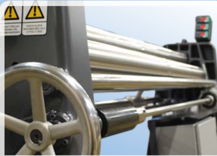
Cone bending equipment, includes diagonal setting of bending roll, trailing shoe and handwheel with dial register
