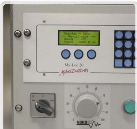
NC control panel
