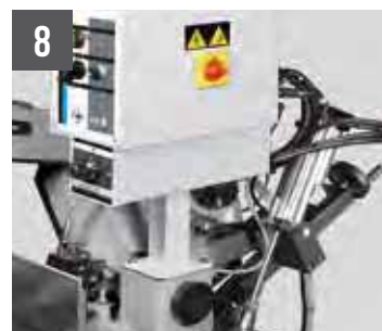
8 SHARK 282 zaagcontrolesysteem (retrofit)
