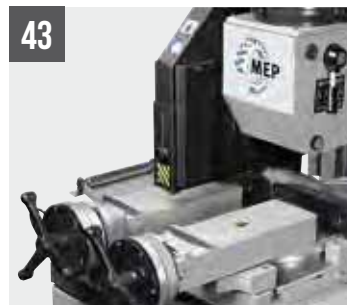
TIGER 352MA/SX EVO/NC 5.0 Extra pneumatische klem
