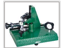
test the effect of lateral force on accuracy of test indicators (half round gage block is required)
