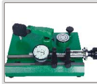
inspect accuracy of dial indicators (range 0-25mm)
