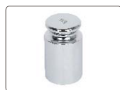
calibration weight (included in 8301-300, 8301-600 and 8301-1200)
