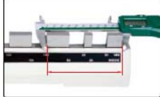
check lower jaws of caliper
