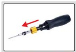
step 3: release the lock ring
