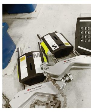
FIXTURLASER EVO - COMPLETE SYSTEM Weight (incl. all standard parts): 4,8 kg (10,6 lbs)
