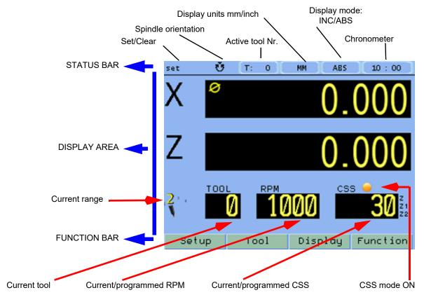
When the spindle is off, the RPM and CSS displays show the programmed values.
