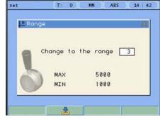
The DRO generates digital outputs in order to be able use an automatic gear change.
