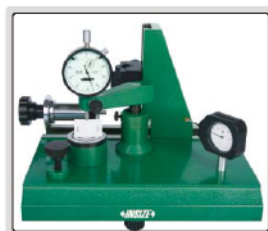
Test repeatability of dial indicators
