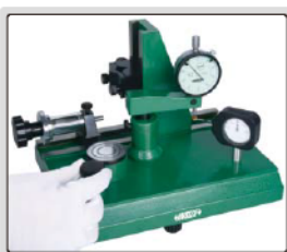
Test force of dial indicators
