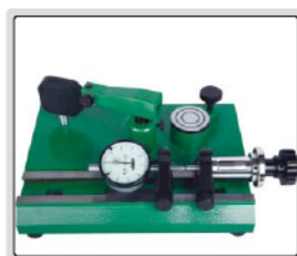
Inspect accuracy of dial indicators (range 0-25mm)
