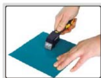
step 1: make grid cutting on surface
