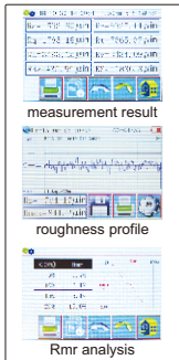
data can be sent to Excel by connecting to computer via bluetooth or USB cable
