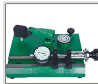
Inspect accuracy of dial indicators (range 0-25mm)
