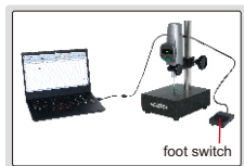
data transmitted to Excel without software
