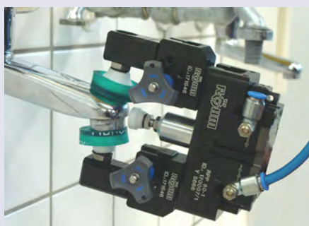
Gripper RPP 80-1 for the leak test of taps
