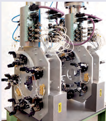
Gripper changing station with 20 integrated RZP-grippers
